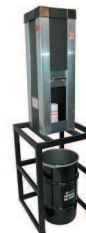
HDC-150-94 Heavy Duty Truck Filter Crusher -Height 40" -Filter Diameter 6" -Width 12-3/4" -Crushing Force 15 tons -Depth 12-3/4" -Pump Type: Air/ -Filter Height 7-1/2" Hydraulic
